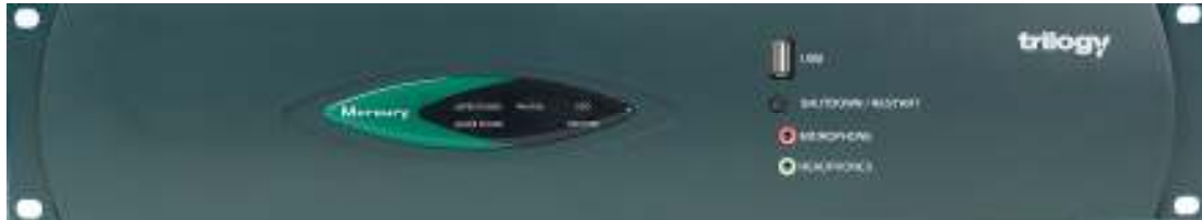
Photo caption – A Mercury Interface Unit (MIU), the device used to tie all of the sites together over an IP network
