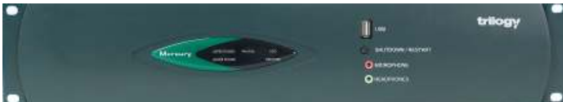
Photo caption – A Mercury Interface Unit (MIU) used to connect multiple sites using IP over an ADSL network.
