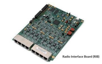
The Radio Interface Board (RIB) is an optional card that interfaces with up to eight half-duplex and/or full-duplex radios.
