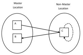
In the scenario depicted here, if Panel A is speaking to Panel C, then when Panel C speaks to Panel B, it is the route from Panel A to Panel C that is dimmed.
