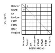
**Mirror dimming.** This term is derived from the traditional crosspoint diagrams that were used to depict talkback systems. Sources and destinations provide the axes of an X-Y grid, and symbols are used to depict crosspoint at the intersection of a source and destination.
