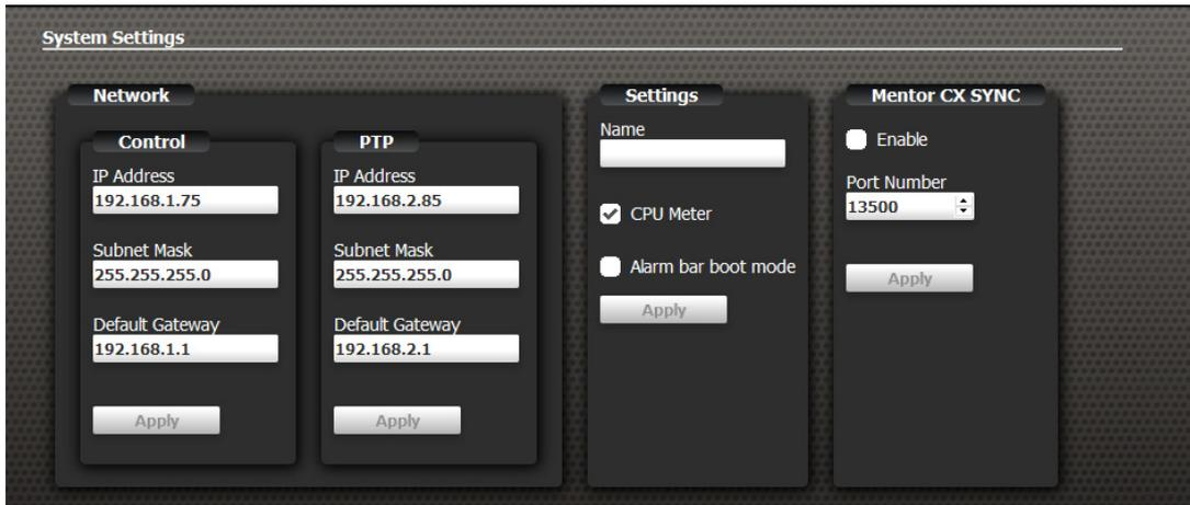
Mentor RG network settings can be changed here: remember that if you change the network address to a different subnet, you may lose contact from your current PC address.
