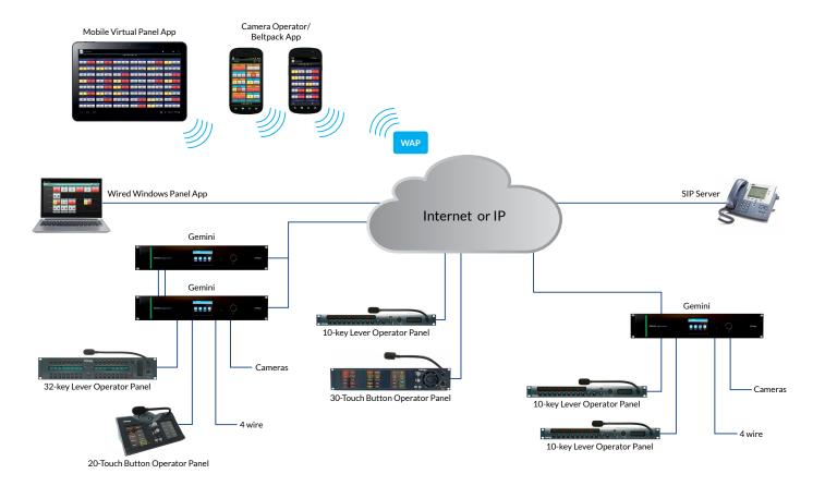
NOTE: The Trilogy Virtual Panel requires an SIP-enabled Trilogy matrix with DSP to operate.
