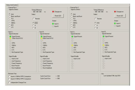
**Channel Pair x** – This box contains the controls and status of the inputs of each channel pair.
