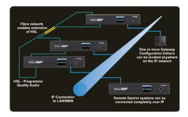
It also supports a further 64 communication channels over IP, and the integral audio mixer/DA allows up to 12 channels of camera intercom to be connected without using standard audio ports.
